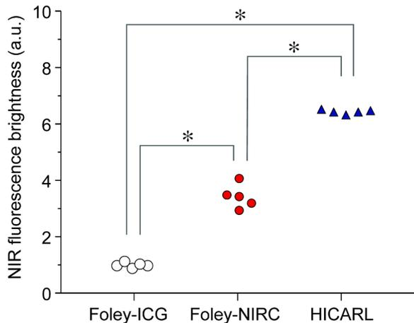
**Fig. 3.** Graph showing NIR fluorescence brightness of the Foley-ICG catheter (white filled circles), Foley-NIRC catheter (red filled circles), and HICARL catheter (blue filled triangles) during irradiation of excitation light. The average value of NIR fluorescence brightness of the Foley-ICG catheter was scaled to 1. \* $p < 0.05$ ,  $n = 5$  for each group. a.u., arbitrary units.
