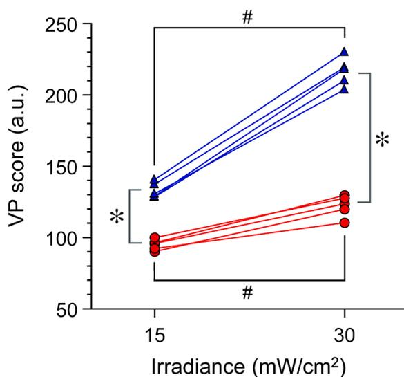
Fig. 5. Graph showing visibility performance (VP) score of the Foley-NIRC catheter (red filled circles) and HICARL catheter (blue filled triangles) during weak (15 mW/cm<sup>2</sup>) and strong (30 mW/cm<sup>2</sup>) irradiation of excitation light. \**p* < 0.05, *n* = 5 for each group; #*p* < 0.05, *n* = 5 for paired samples. a.u., arbitrary units.
